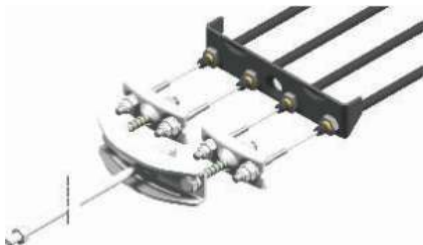
An example for mounting the old version of brake cables for tandem axle
